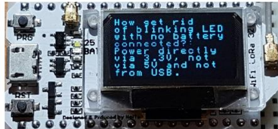
Figure 1.1 Ecran OLED de la carte ESP32 (Heltec WiFi LoRa 32)
