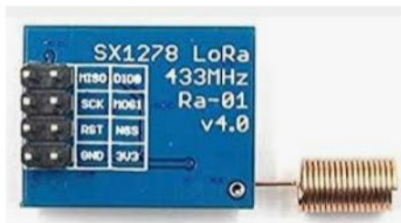
Fig 4.1 The LoRa modem-module (Ra-01) with its SPI connector
